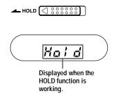
You can use the HOLD function with both the CD player and remote control. You can still operate your CD player using the remote control when HOLD on the remote control is set to off
